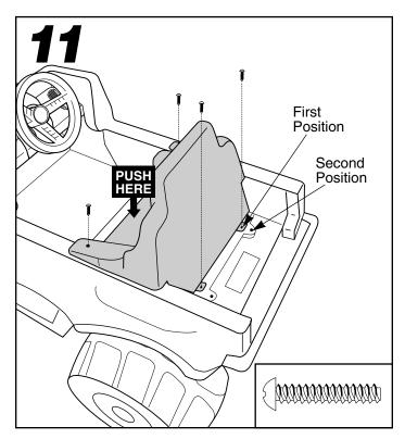
**Note:** The seat can be assembled in either of two positions for your child's comfort.
